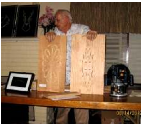
Here he explains how he uses pattern boards and a v-groove router bit to get the effects shown above.
